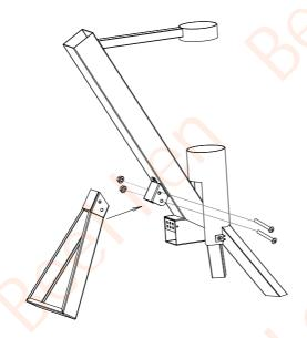
Step4, Insert the support leg 2 into the rocket body support and tighten with long screws and bolts (pay attention to the level adjustment).
